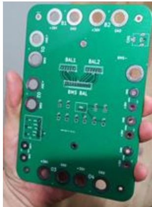
Power Distribution PCB
