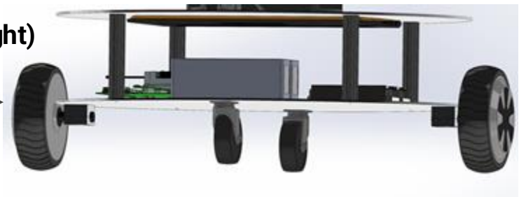
4 x 2020 T-Slot Supports on 11ga Aluminum Plates
