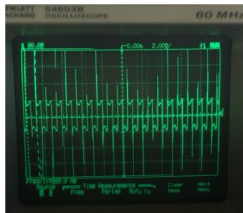
Figure 9. Frequency continued to increase until the end of the sweep (15,000 Hz) was reached. Amplitude had eventually reduced as well.
